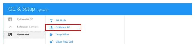
**3** A dialog appears prompting you to enter the SIT Lift Distance. Enter the distance, then click **Calibrate SIT**. The lift distance is the distance in millimeters from the tip of the SIT to bottom of the well.
