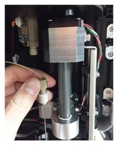
**9** Verify that the tubing contacts the bottom of the tube on the SIP.
