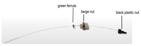
**3** Open the SIT door. Identify the three components shown in the following figure.
