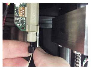
**5** Follow the tubing from the black nut down to the beige plastic nut. Twist off the beige nut and gently pull it and tubing out from the SIP.
