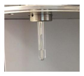
**10** Secure the black nut to the bottom of the flow meter so it is firmly attached. Make sure the sample line bends away from the SIT assembly when the SIT stage rises.
