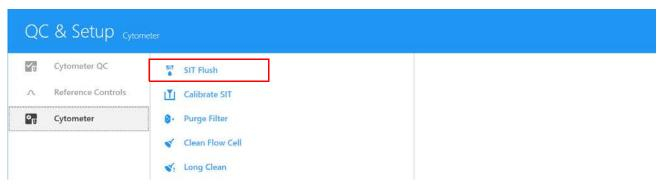
2 If carryover or a clog persists, place a tube of 10% bleach on the SIP and acquire at High flow rate for 5 minutes. Afterwards, acquire a tube of DI water at High flow rate for 5 minutes.
