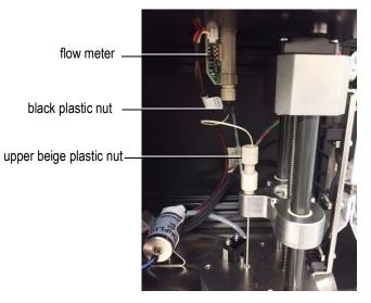
4 Twist off and carefully remove the black plastic nut from the bottom of the flow meter.
