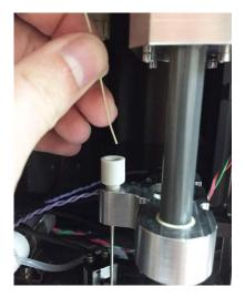
8 Once the line is in, screw in the beige nut until finger tight. You will feel once the nut is secured to the bottom.
